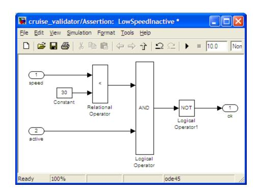
"If speed is < 30, cruise control must remain inactive"
